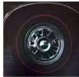
High speed 7.50 x 14 nylon tires were designed specially for the GTO, mounted on 14 x 6.75 wide rims. This is the optional deluxe wheel cover.
